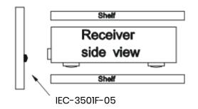
IR emitter is attached to rack door,round shape side facing the IR window
